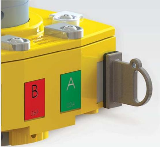
Removal of a key from the assembly increases the scope for the ingress of dust and dirt through the key entry aperture which can contaminate the inner workings of the lock mechanism - leading ultimately to possible seizure and malfunction.
